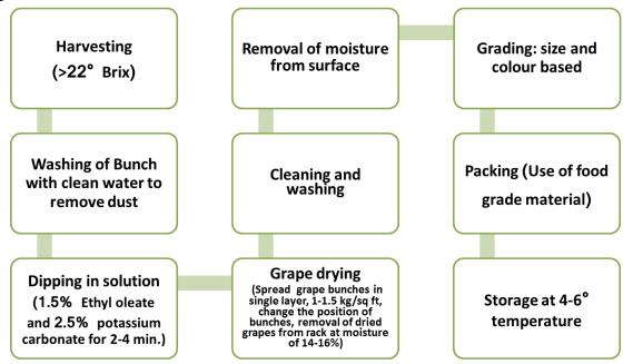
Fig.1 Diagram of grape drying process
