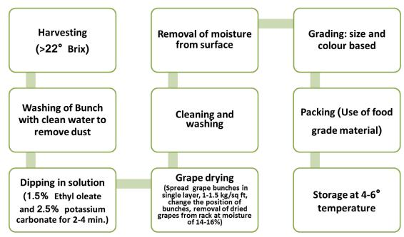
Fig.1 Diagram of grape drying process
